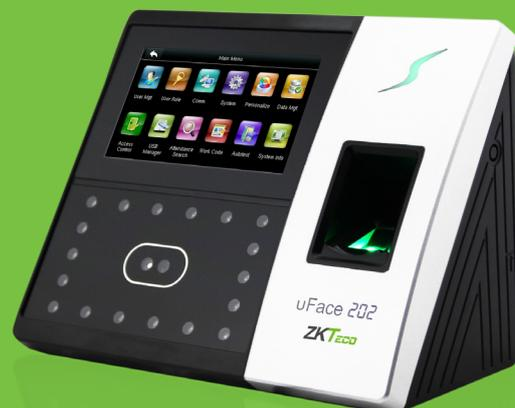
ZKTeco has released the uFace202 Multi-Biometric T&A and Access Control Terminal which supports 3,000 face templates, 3,000 fingerprint templates and 10,000 cards. It is equipped with ZKTeco latest hardware platform and algorithm, which provide clients with a brand new UI and user-friendly operating interface, bringing them a smooth using experience. With the advanced face algorithm and multi-biometric verification technology, the terminal's security level of verification is greatly enhanced.
